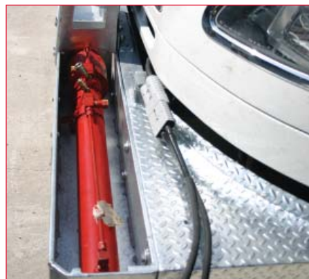
Hydraulic cylinder in horizontal position, from left side of truck, inside front bumper
