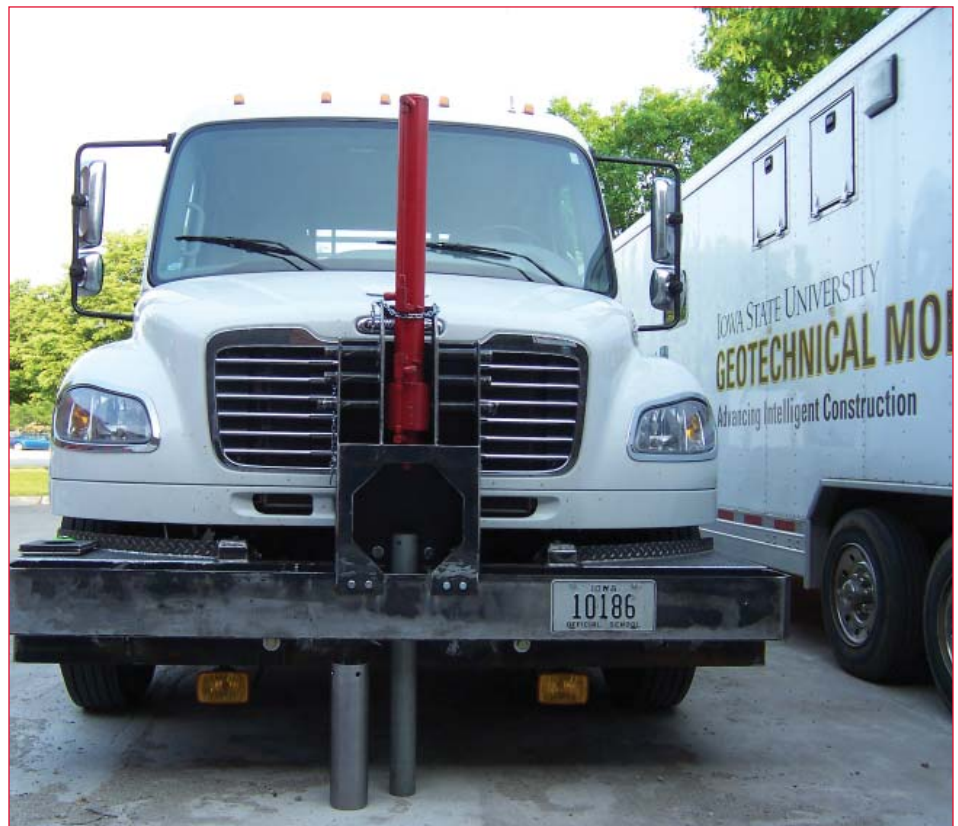
Hydraulic tube sampling device attached to the front of the Freightliner truck
