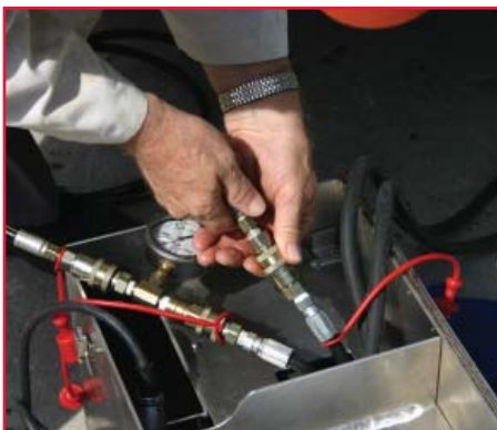
Operator attaching hydraulic power unit using quick-couplings
