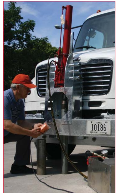
Hydraulic cylinder and Shelby tube in sample collection configuration
