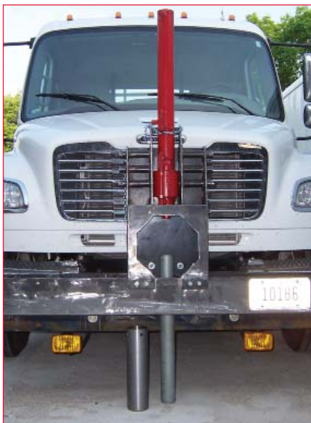
Hydraulic cylinder and Shelby tube, vertical position
