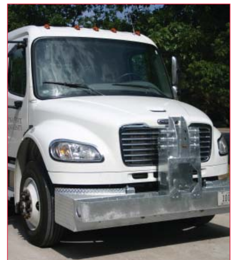
Modified bumper and mounting frame assembly
