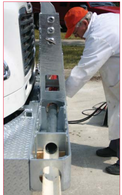
Shelby tube and extrusion support in sample extrusion configuration
